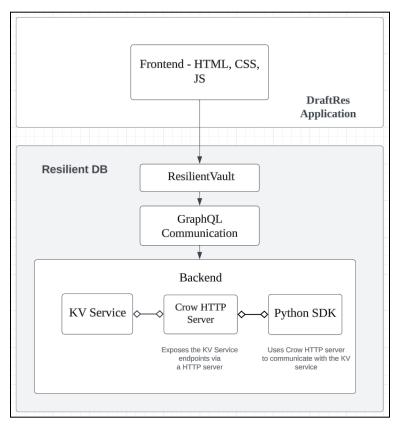
Fig. 2. System Architecture
